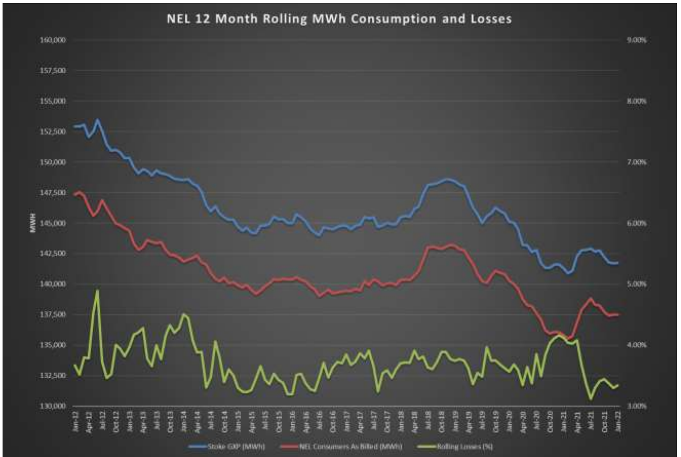
Figure 2: Nelson Electricity Historical GXP and Billed Consumption MWh
